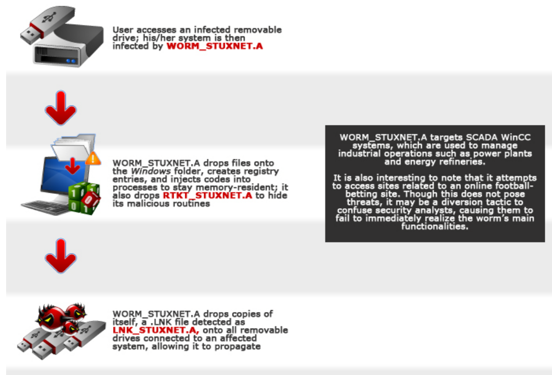
Figure 16 – WORM_STUXNET.A infection diagram (Trend Micro Incorporated, 2010)
